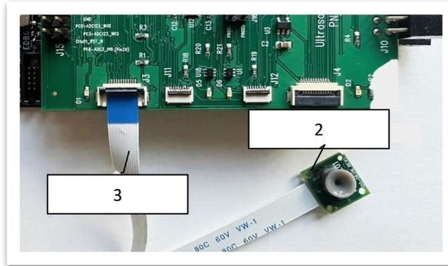
2. Up to 4 sensors can be attached to the connectors on the daughter board using the flat flex cable. Place the unit flat on the module holder, adjust the target to be approximately 300 mm from the sensor. Keep the surrounding area of the fixture clear to avoid any possible interferences. The image below shows the physical connections to run the Module Test software.
