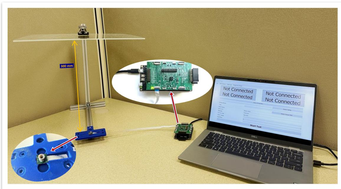
3. Plug the Micro USB connector to J8 of the Development board while the other end of the cable should be connected to host PC.
