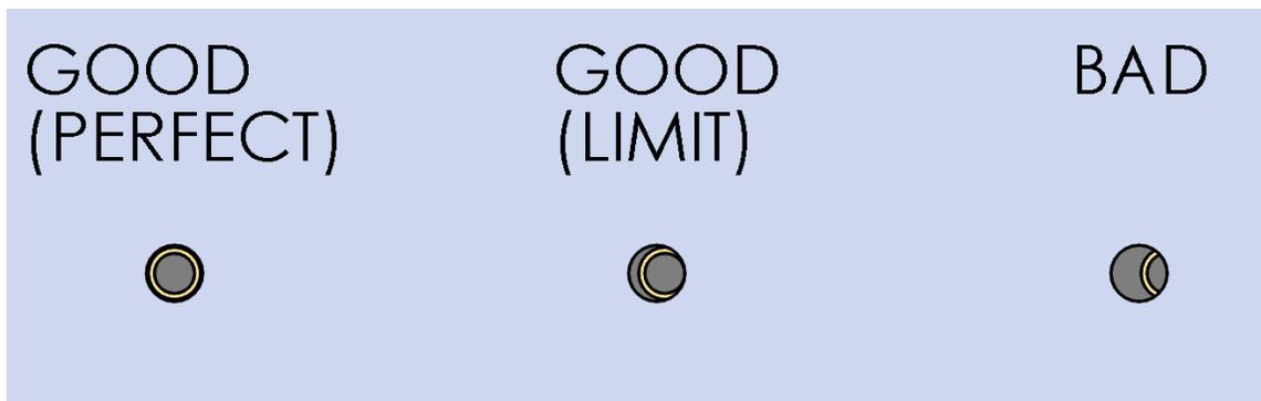
**Figure 17. Examples of various degrees of sensor port alignment with the Acoustic Interface, from perfect concentric alignment (left), maximum acceptable limit tangent alignment (middle), to bad occluded alignment (right).**
