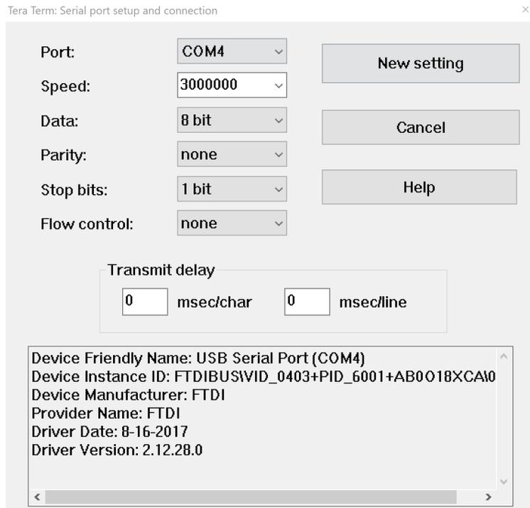
**Figure 3. Serial Port Setup and connection**
