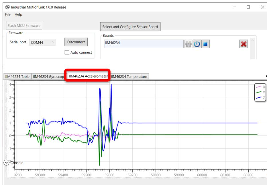
**Figure 26. Graphical representation of Accelerometer Values**
