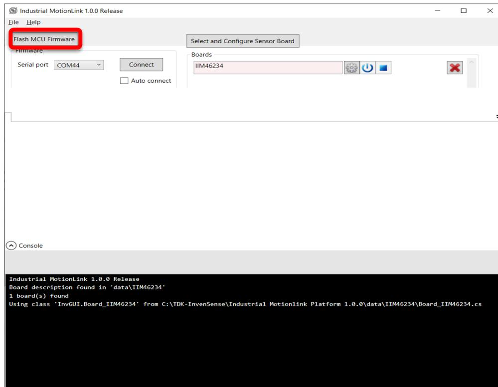
**Figure 18. Flashing the MCU Firmware**
