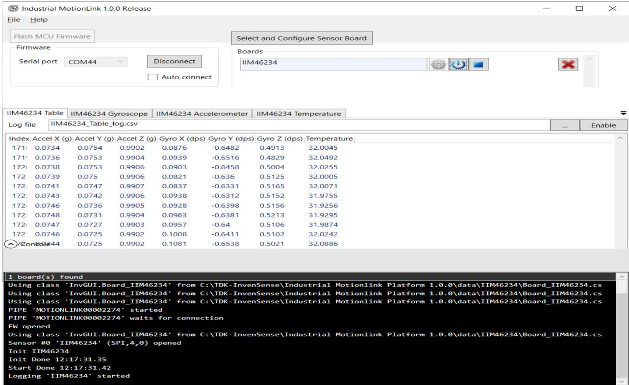
**Figure 24. Combined tabular representation of Accel, Gyro, and Temperature data**
