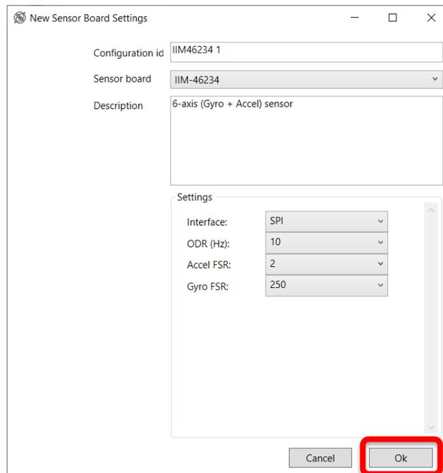
Figure 20. Configuration of Sensor Board
