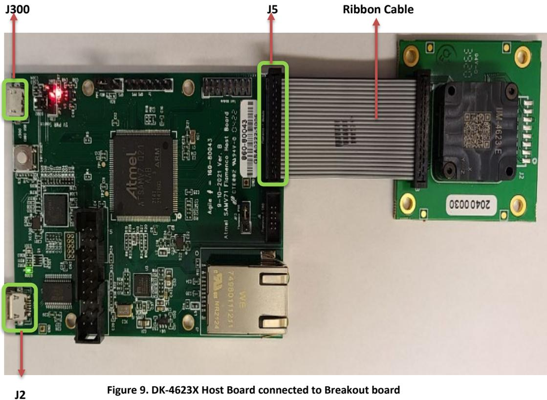
Figure 9. DK-4623X Host Board connected to Breakout board
