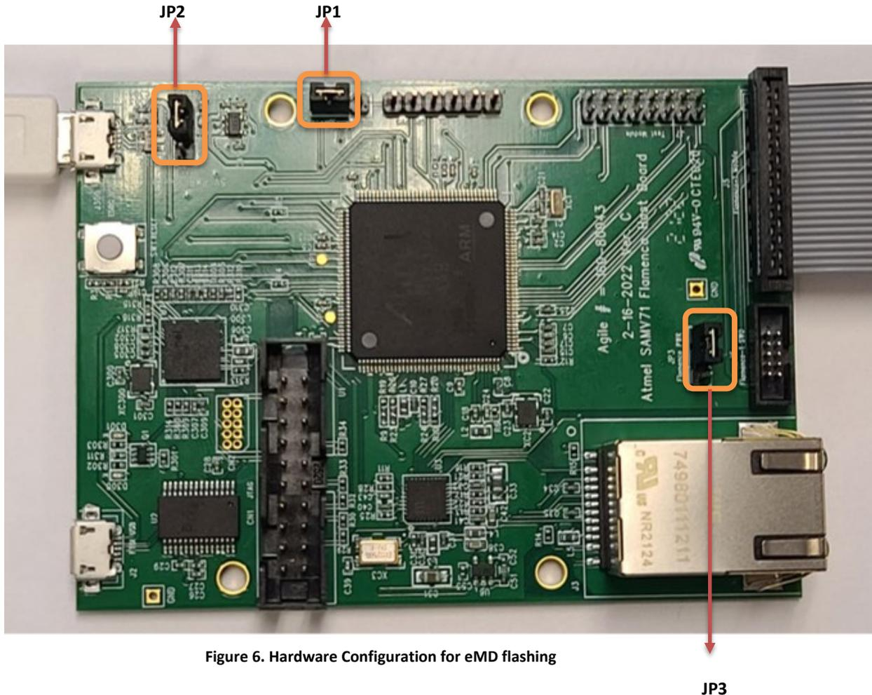
Figure 6. Hardware Configuration for eMD flashing
