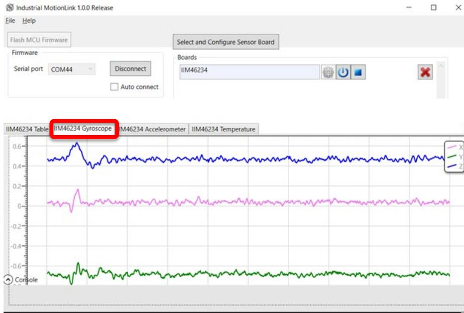
**Figure 25. Graphical representation of Gyroscope Values**
