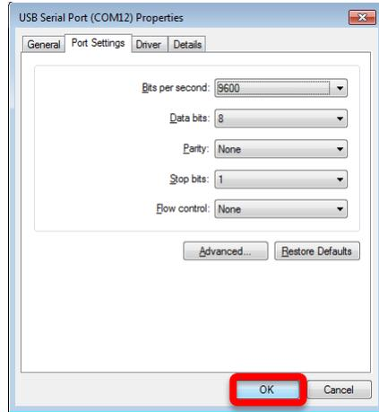
**Figure 33. USB Serial Port Properties**
